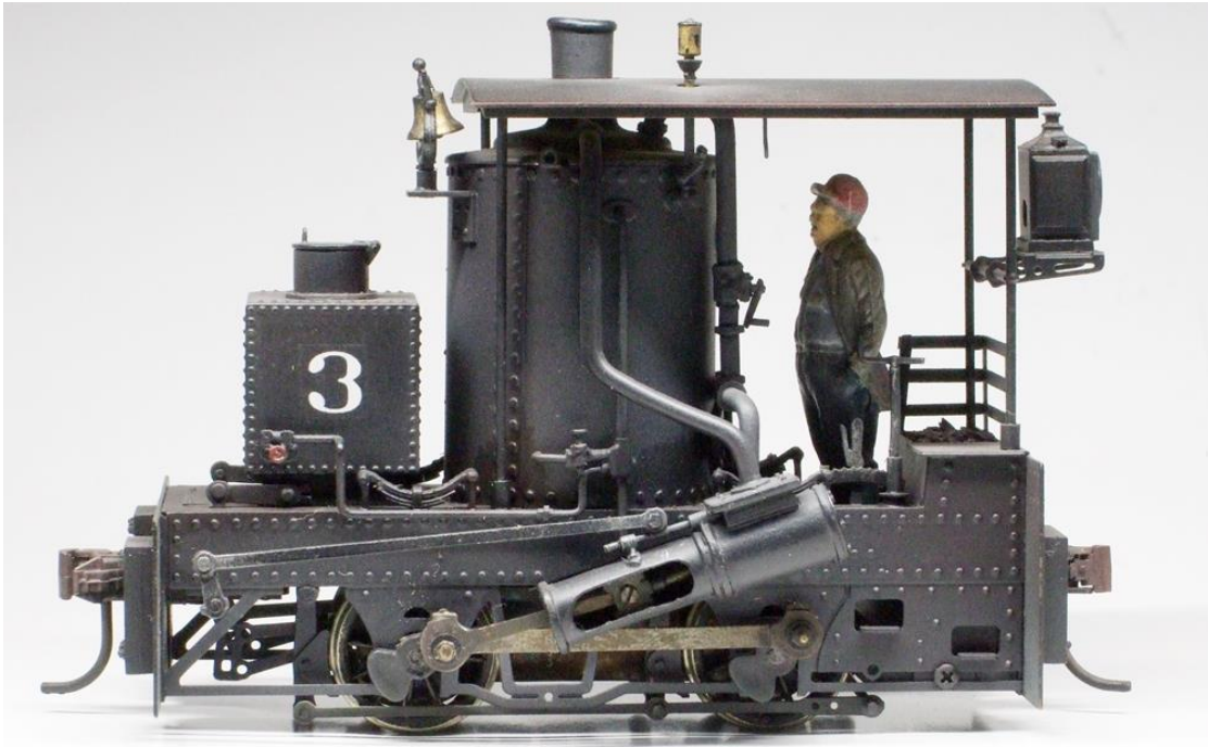
Mortor and DCC sound decorder(Micro Tsunami) , both are inside a vertical boiler
